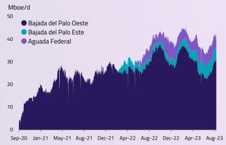
Includes all wells in Bajada del Palo Oeste, Bajada del Palo Este and Aguada Federal normalized to a standard well design of 2,800 meters lateral length and 47 completion stages well
